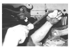
5. Remove bolts from inside cup.6. Add bump stop extension to cup and reattach with longer bolts.
