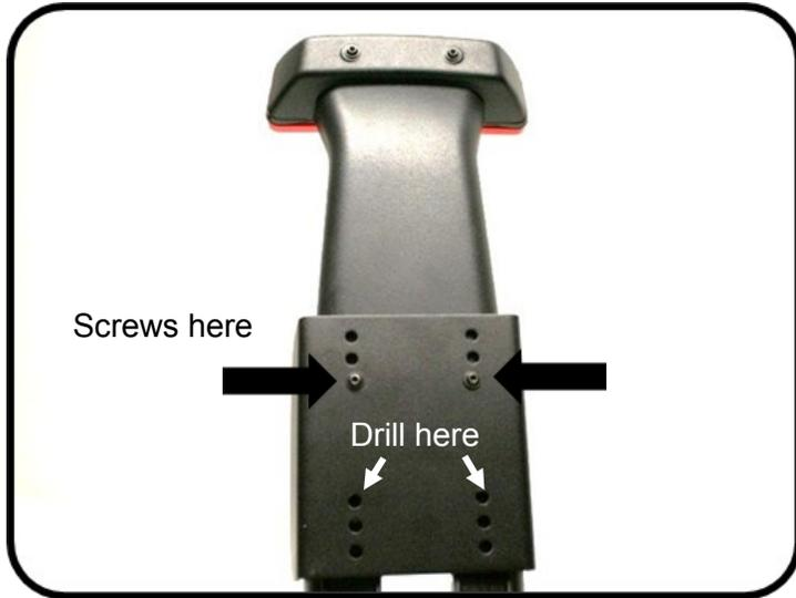
6. Using the extension bracket as a template, drill two 1/4" holes in the tire mount. Use the holes closest to the center of the extension bracket.
