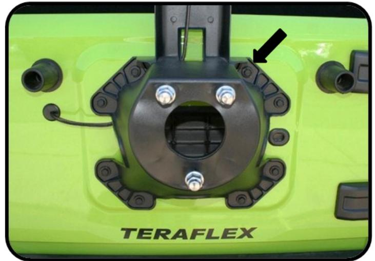
4. With the mount removed, grind off the small bump on the back of the mount.
