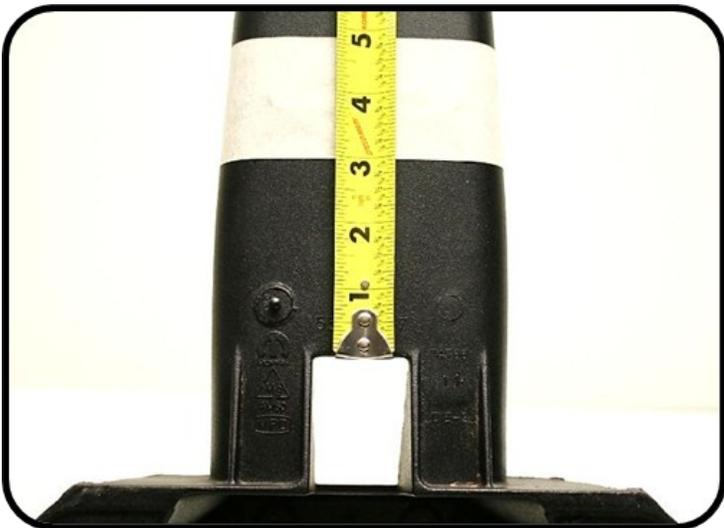
9. Cut along the lower edge of the masking tape using a cut-off wheel.
