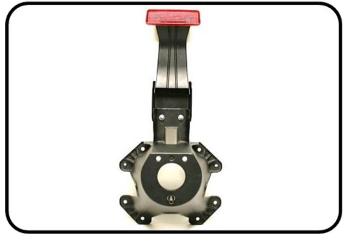
12. Re-install the tire mount onto the tailgate.
