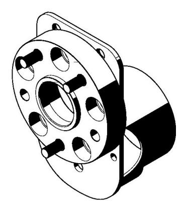
3. Install your spare tire and torque to 60-80ft. Lbs. Your installation is complete.
