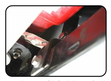
Note: There is some "play" in the bumper after all the bolts are installed and finger tight. This is to allow room for slight variations in mounting points from Jeep to Jeep. Visually inspect the bumper and adjust and align if needed.
