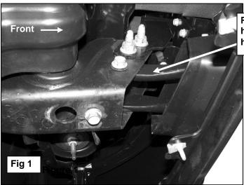
Remove the factory tow hook and hardware. Tow hook will not be reinstalled
