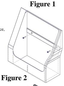
4. Install the Cubby Cover into the plastic cubby by slipping the lower flange into the cubby and lowering the Cubby Cover until the upper flange rests on the outer face of the cubby.(See Figure 3)
