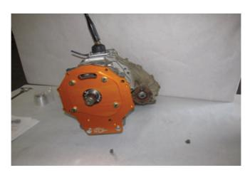
**STEP 12**Install provided coupler to transmission
