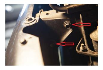
**STEP 3**Unbolt and remove tow hooks.
