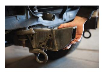
**STEP 4**Slide on bumper an install with supplied hardware.
