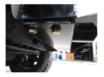
**STEP 2**Slide off stock bumper and remove bumper horns
