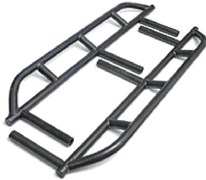
1) Using jack stands, place sliders at desired position on vehicle. Center bars front to rear between wheel openings. Tilt bars up approximately 15 degrees but make sure that both doors will open without hitting the bars.
