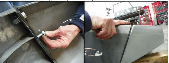
Align flush with the outside of the bumper, and tighten down snug. You do not need to attach the braces yet.
